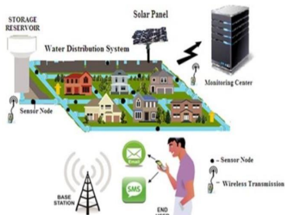
Fig1. Water Distribution Networks Using Wireless Sensor networks
